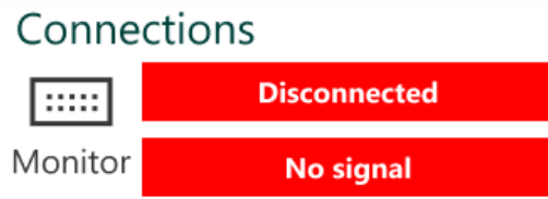
Figure 37: Alert displayed when no signal from blood pressure monitor is detected
