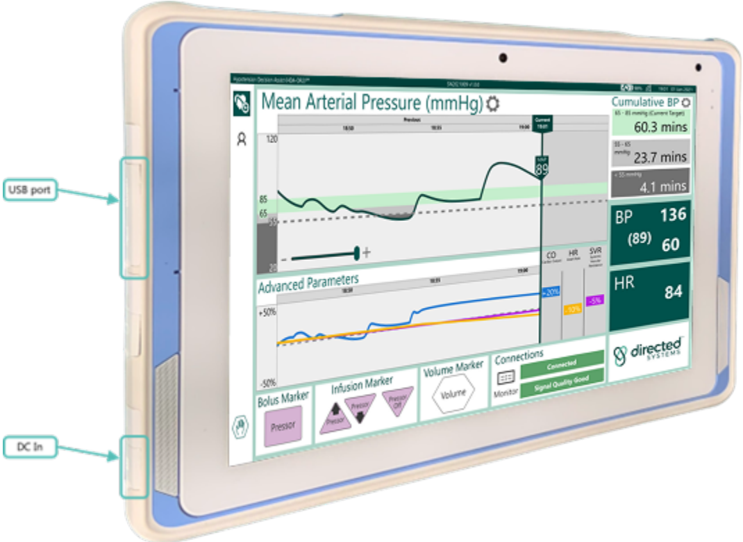
Figure 8: Inputs and Outputs on Advantech Medical Computer
